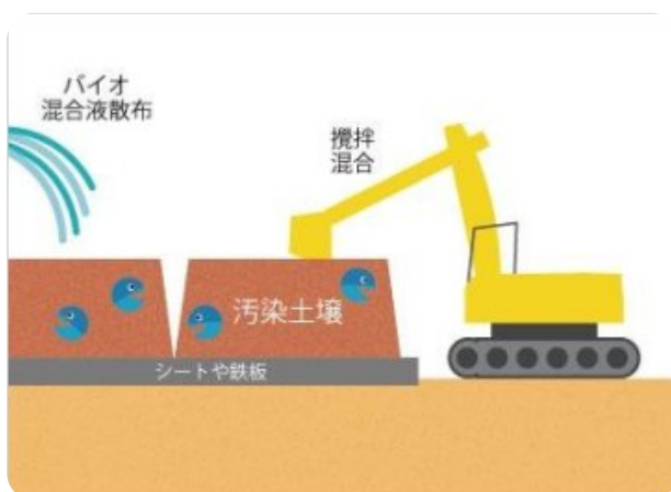
Landfarming: excavated soil is piled up and stirred to mix it
